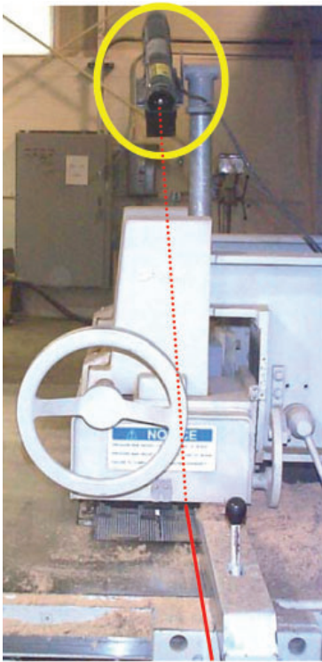
Figure 22.—A laser projection unit mounted above a straight-line rip saw projects a laser line onto boards placed on the infeed table enabling the rip saw operator to see where the sawline will fall on the board.
