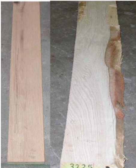
Figure 8.—Split, stain, and wane defects that run for some distance along the length of the board are best removed in a rip-first operation.
