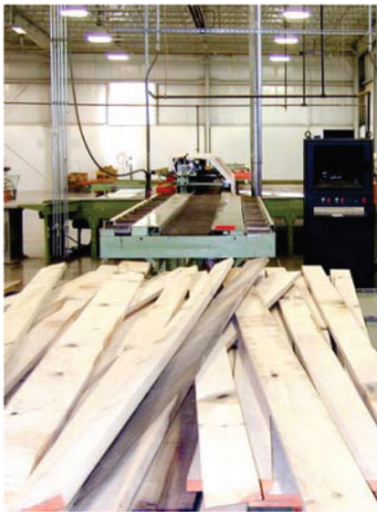
Figure 31.—Boards piled up at marker station cause the person doing the marking to spend time and energy straightening them out before they can be pulled into marking position.
