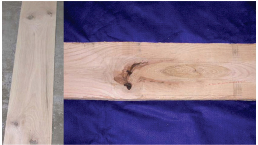
Figure 9.—Defect clusters and large defects that occupy a significant cross-section of the board are best removed in a crosscut-first operation.
