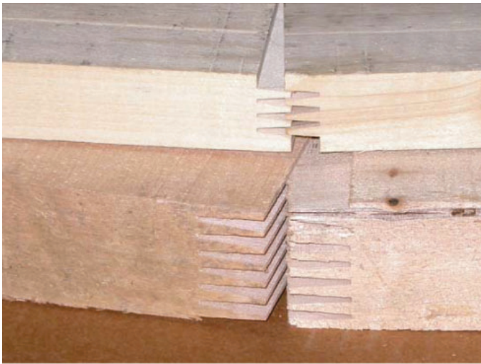
Figure 39.—Two sets of fingerjoint blanks that show how joint length can vary.
