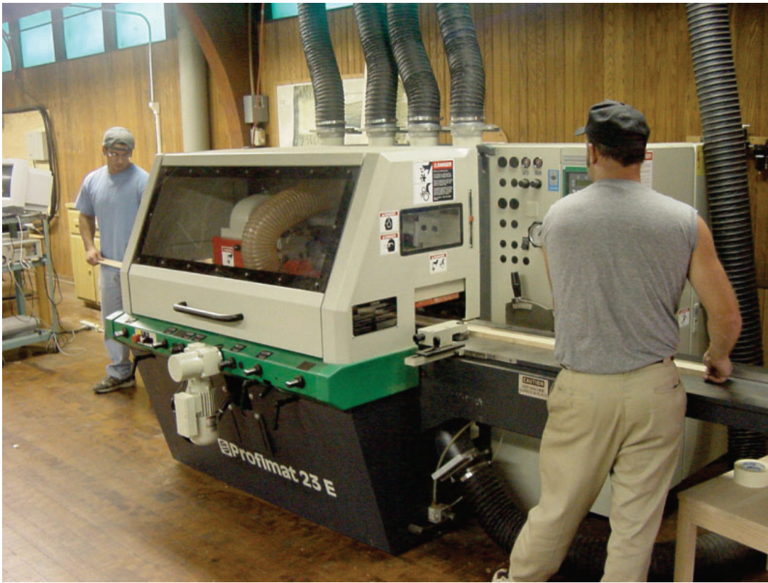
Figure 41.—A manual feed, mid-size, four-head moulder.
