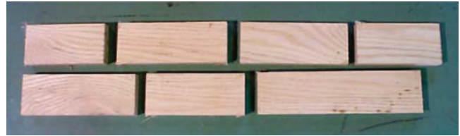
Figure 38.—Fingerjoint blocks are recovered wood sections that are too short to meet length requirements specified in the cutting bill.
