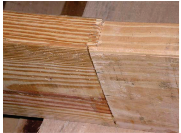
Figure 40.—Nonparallel edges and unequal block widths can lead to offset fingerjoints that generally must be rejected.
