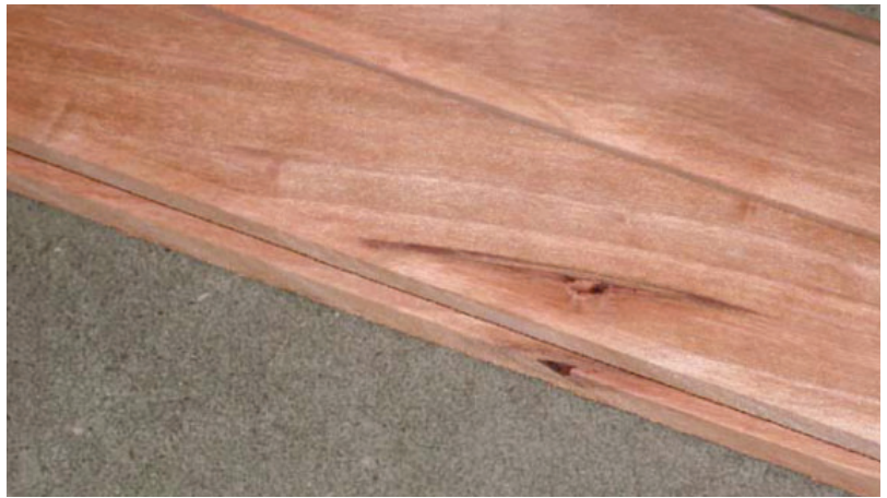
Figure 42.—A moulded piece in which a hidden defect in the wood was exposed by the moulder machining process causing the piece to be rejected.
