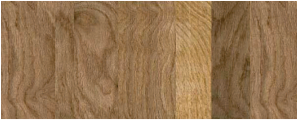
Figure 35.—An example of a panel in which the component parts are poorly matched in terms of color and grain pattern.
