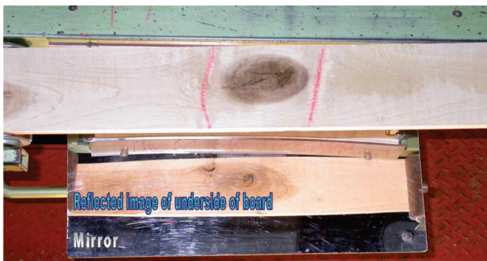
Figure 28.—The view of both the top and underside of a board as seen by the defect marker using a well positioned mirror.
